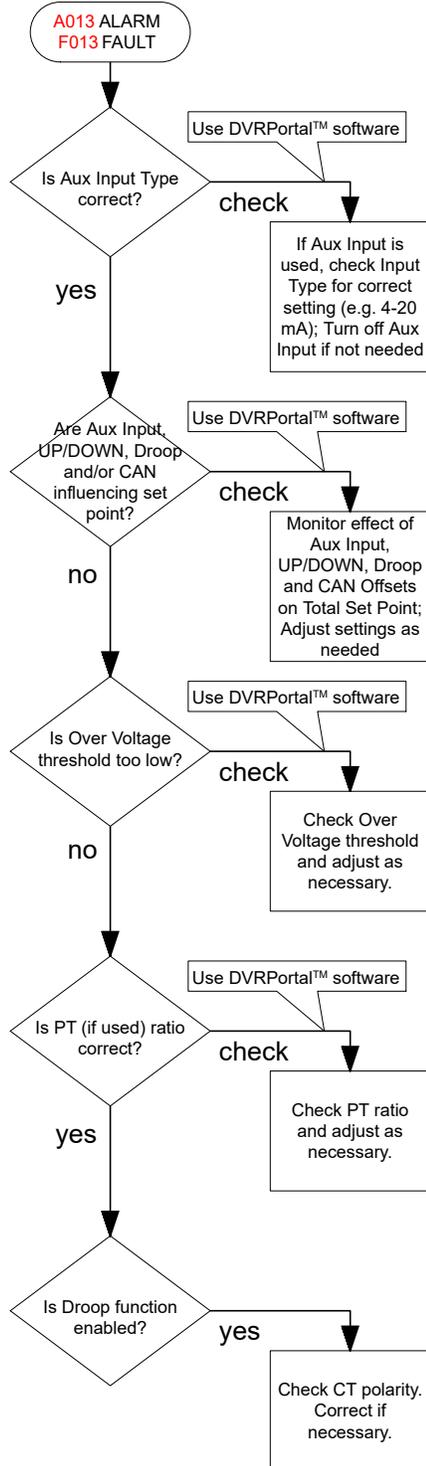
**Reverse Power Flow Alarm/Fault**
