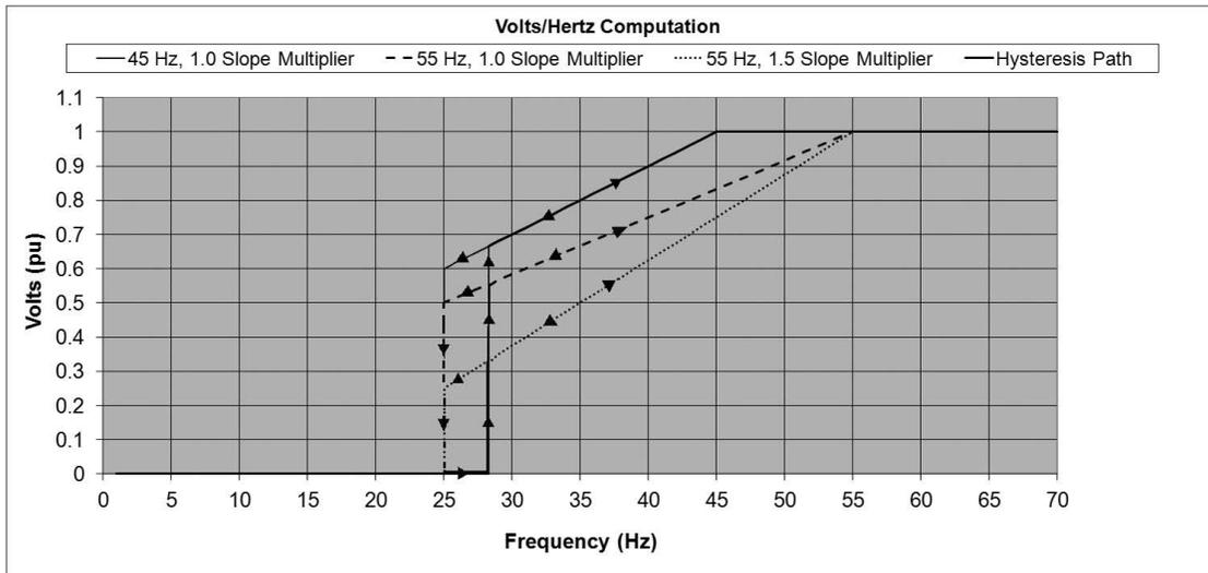
Figure 4-4. Examples of Under Frequency and Slope
