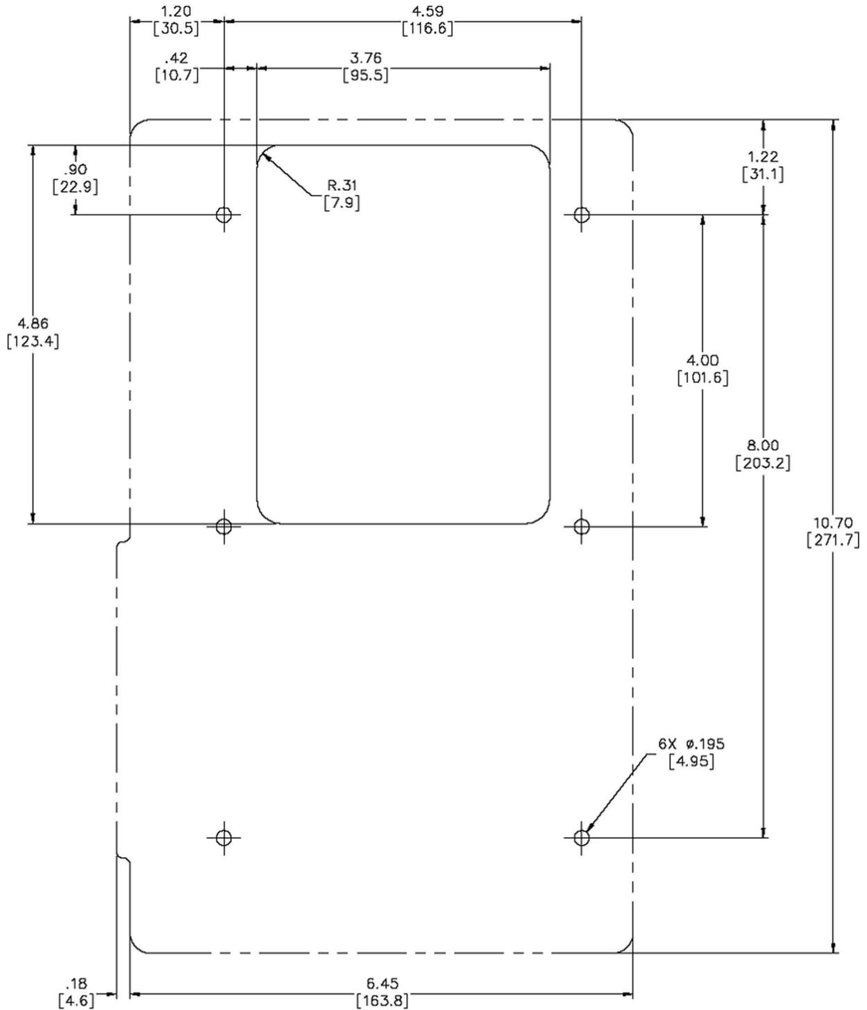
Figure 5-3. Cutout and Drilling Dimensions. Valid for 2400 & 2500 versions.
