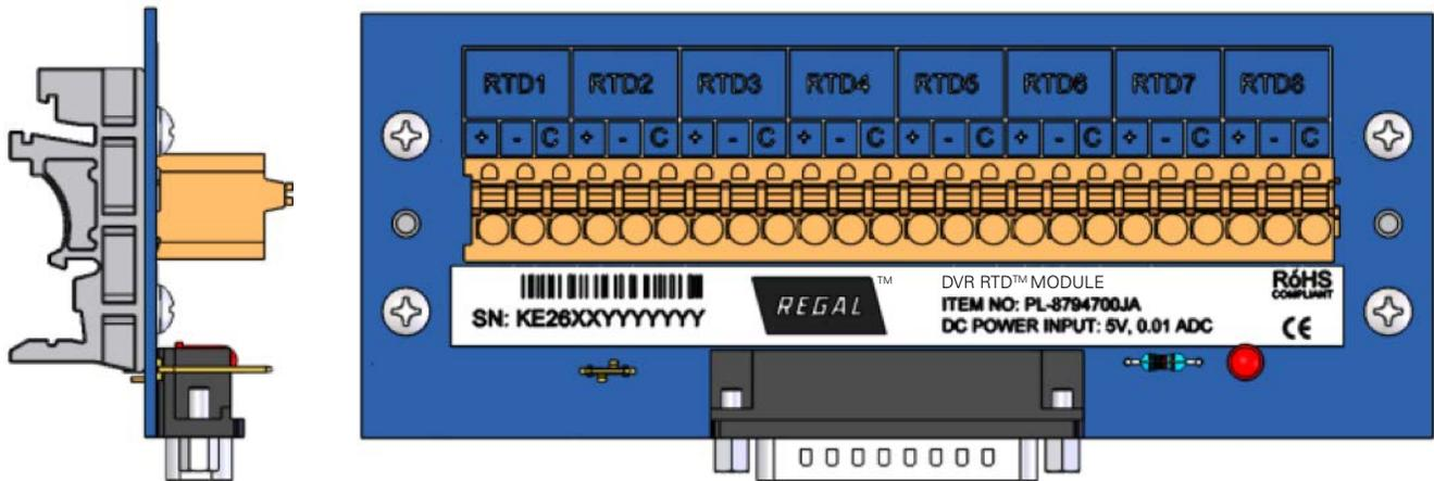
**Note:** Loctite<sup>®</sup>\* 242 or similar should be used on the screws before connecting the DB25 cable to the RTD module and DVR<sup>®</sup> regulator for better vibration withstand. Recommended torque is 7.0 inch-lbf [0.8 N-m].
