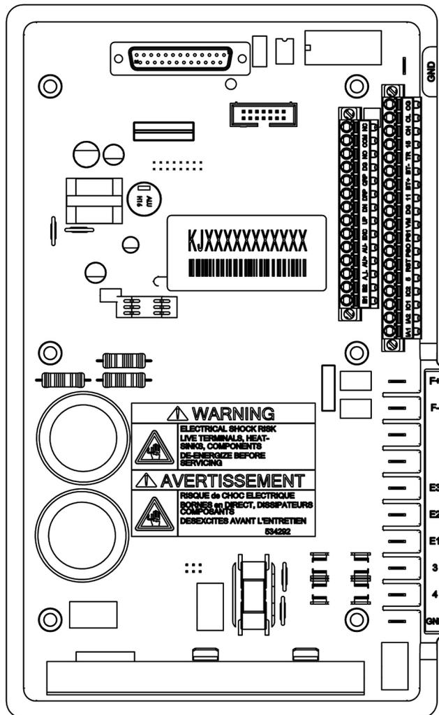
Figure 5-4. The regulator Rear Panel Connectors (DVR<sup>®</sup>2500 regulator shown)
