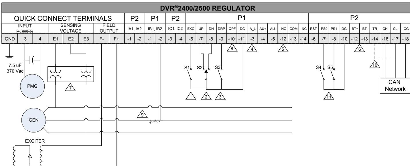
Figure 5-9. Typical Connections to a Single-Phase Generator
