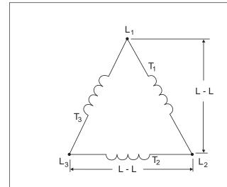
Three lead generators have 3 coil groups with one end of each group connected into a Delta internally. There are 3, 6, or 12 cables or 3 bus bars coming out of the generator.
