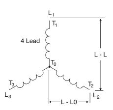
Four lead generators have 3 coil groups with one end of each group connected together. There are 4, 8, or 16 cables or 4 bus bars coming out of the generator.
