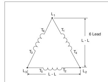
Six lead generators have 3 coil groups with 6 or 12 cables coming out of the generator.
