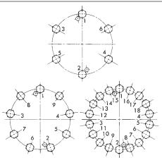
Torque the bolts in the above sequence according to the correct bolt pattern.
