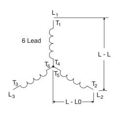
Six lead generators have 3 coil groups with 6 or 12 cables or bus bars coming out of the generator.
