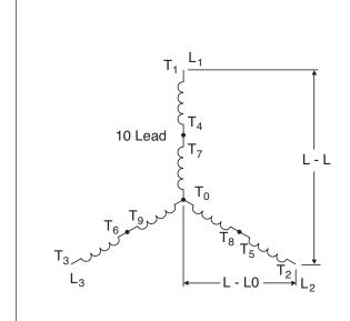
Ten lead generators are dual voltage generators with six coils. One end of the three inner coils is connected together. There are 10 or 20 cables coming out of the generator.
