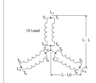
Twelve lead generators are dual voltage generators with six coils which don't have the connection of the three inner coils. There are 12 or 24 cables coming out of the generator.
