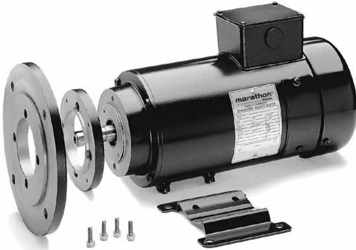
*Three common IEC mounting options are shown in this photo. From left, a B5 flange, B14 face and rigid B3 base. In this case, any of the options can be bolted to a modularly designed round-body IEC 71 frame motor.*
