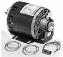
**Resilient base** has isolation or resilient rings between motor mounting hubs and base to absorb vibrations and noise. A conductor is imbedded in the ring to complete the circuit for grounding purposes.
