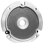
**NEMA D flange mount** is a machined flange with rabbet for mountings. Bolts pass through motor flange to a threaded hole in the mounted part. NEMA C face motors are by far the most popular and most readily available. NEMA D flange kits are stocked by some manufacturers, including Marathon Motors.
