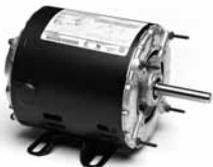
**Extended through-bolt** motors have bolts protruding from the front or rear of the motor by which it is mounted. This is usually used on small direct drive fans or blowers.
