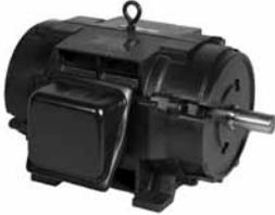
**Open Drip Proof (ODP)** motors have venting in the end frame and/or main frame, situated to prevent drops of liquid from falling into the motor within a 15° angle from vertical. These motors are designed for use in areas that are reasonably dry, clean, well-ventilated, and usually indoors. If installed outdoors, ODP motors should be protected with a cover that does not restrict air flow.
