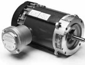
**Explosion Proof** motors meet Underwriters Laboratories or CSA standards for use in the hazardous (explosive) locations shown by the UL/CSA label on the motor. The motor user must specify the explosion proof motor required. Locations are considered hazardous because the atmosphere contains or may contain gas, vapor, or dust in explosive quantities.
