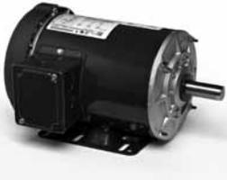
**Totally Enclosed Fan Cooled (TEFC)** motors are the same as TENV except they have an external fan as an integral part of the motor to provide cooling by blowing air over the outside frame.
