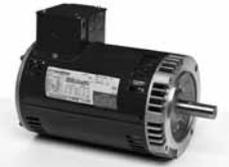
**NEMA C face mount** is a machined face with a pilot on the shaft end which allows direct mounting with the pump or other direct coupled equipment. Bolts pass through mounted part to threaded hole in the motor face.
