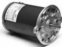
**Type M or N mount** has special flange for direct attachment to fuel atomizing pump on an oil burner. In recent years, this type of mounting has become widely used on auger drives in poultry feeders.
