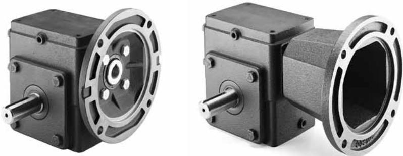
At left, a quill-style input worm gear reducer uses a hollow input shaft and a shallow mounting flange. At right, extended mounting flange accommodates a solid-shaft to solid-shaft input with a flexible coupling joining the two shafts.
