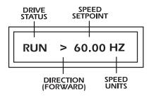
As in the STOP mode, the ENTER key can be used to toggle the display from SPEED to % LOAD to VAC (motor voltage):
