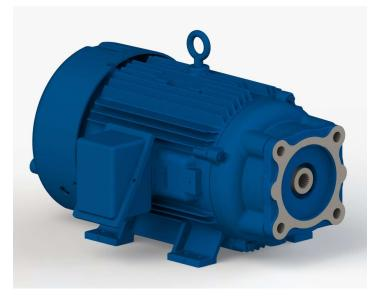
Marathon Electric is excited to announce the introduction of our new Hydraulic Pump Motors. These motors are designed with highly engineered adapter pads allowing the motor flange to mount to SAE A, B, and C flanges for both 2 and 4 bolt configurations. The motor shafts will have a standard SAE shaft configuration that will vary per frame size. Special internal spline adapts can be used to change from one spline configurations to another. Internal keyway shaft extensions will also be available.
